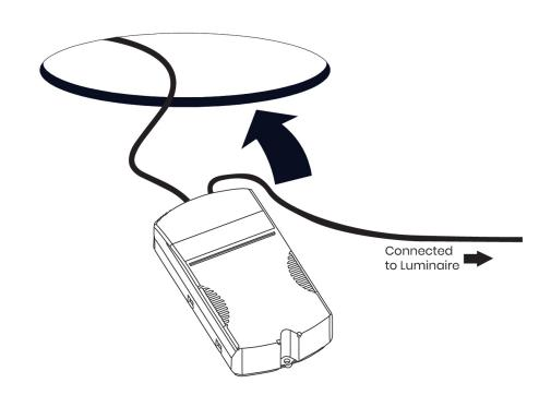
Offer up LED STAR luminaire to ceiling. A push/fold 2 x springs backward, **B** Push luminaire through ceiling cutout, please ensure all springs are evenly pushed through.
