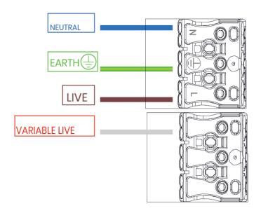
Example switchDIM circuit 220-240 V 0/50/60 Hz
