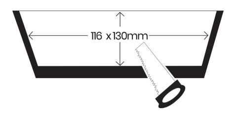
Feed Incoming supply (provided by others) through ceiling cut-out and connect into driver (See pages 6-8 for all wiring diagrams).
