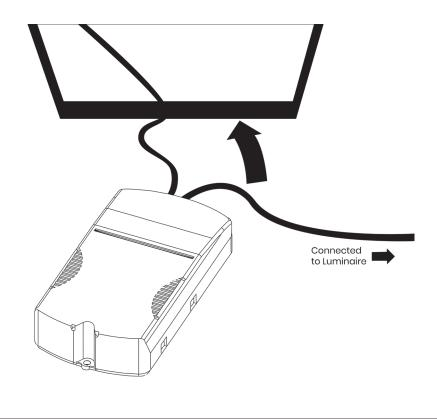
Offer up Quadrina luminaire to ceiling. A push/fold 4 x springs backward, B Push luminaire through ceiling cutout, please ensure all springs are evenly pushed through.
