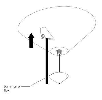
4 Connect luminaire supply to pre supplied connector block.
