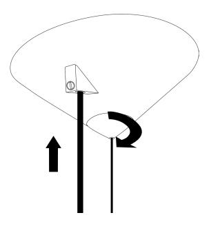
Tighten cable restraint using a flat headed screwdriver (Not supplied).
