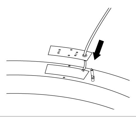
10 Please re-attach the electrical cover plate using the two screws.
