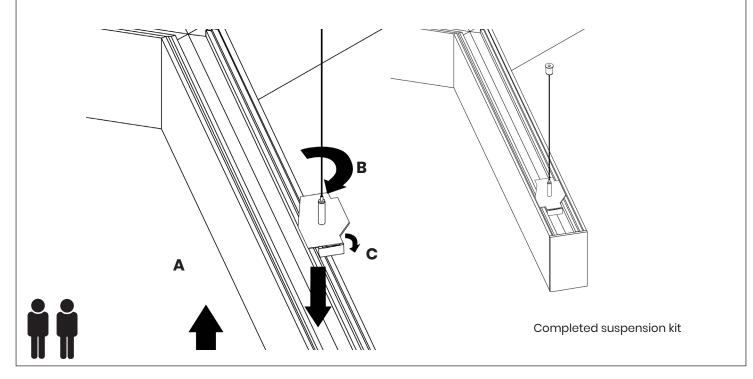
Adjust suspension plates to 110mm from end of bodies. To ensure cable gland is not blocked/covered.
