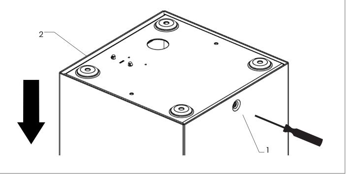
Offer up luminaire to desired surface. Install using appropriate (M5) fixings. (Supplied by others)
