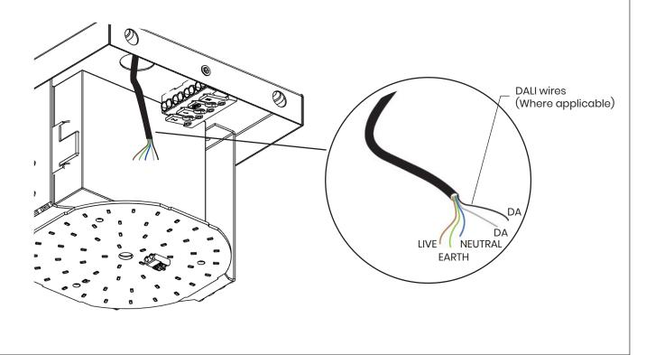
Once incoming supply cable has been connected. Re attach the outer housing using the two M4 countersunk screws.
