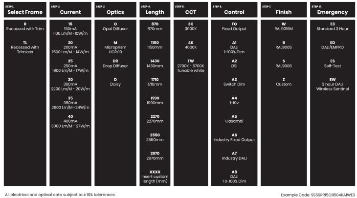
All electrical and optical data subject to ± 10% tolerances. Values based on 4000K Colour temperature.
