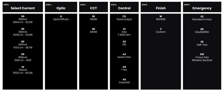
All electrical and optical data subject to ± 10% tolerances. Values based on 4000K Colour temperature and Opal diffuser. Example Code: ULTRALUX50O3KA1WE3
