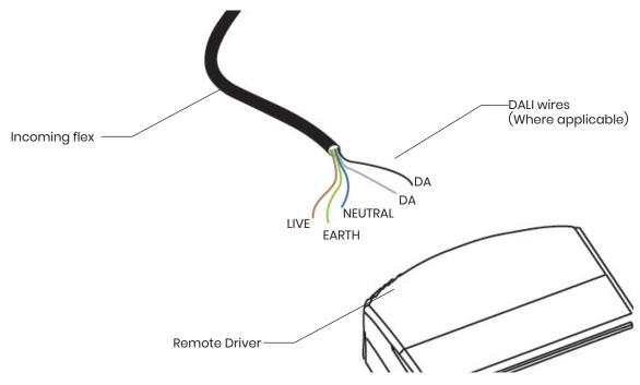
3 Feed driver or driver gear box through ceiling cut out.
