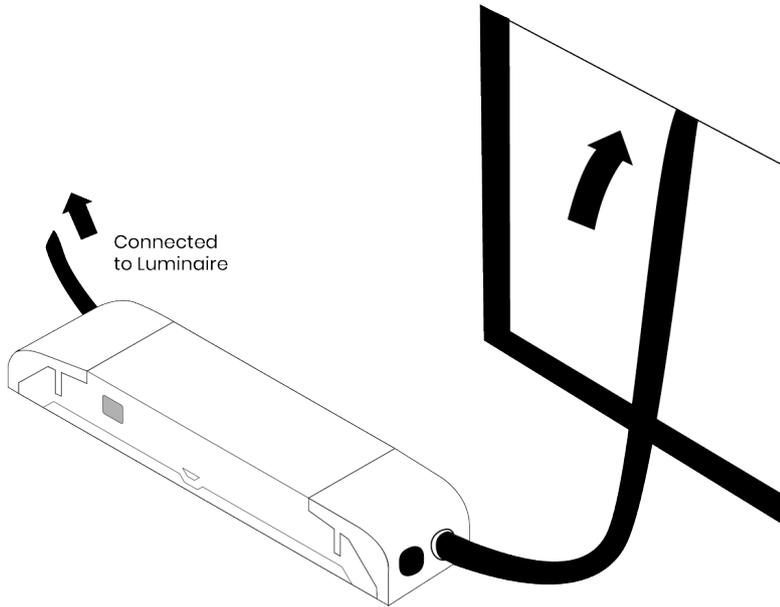
**4** Offer up NL luminaire to void cut-out. **A.** Push/fold 2 x springs backward, **B.** Push luminaire through cutout, please ensure no wires are trapped.
