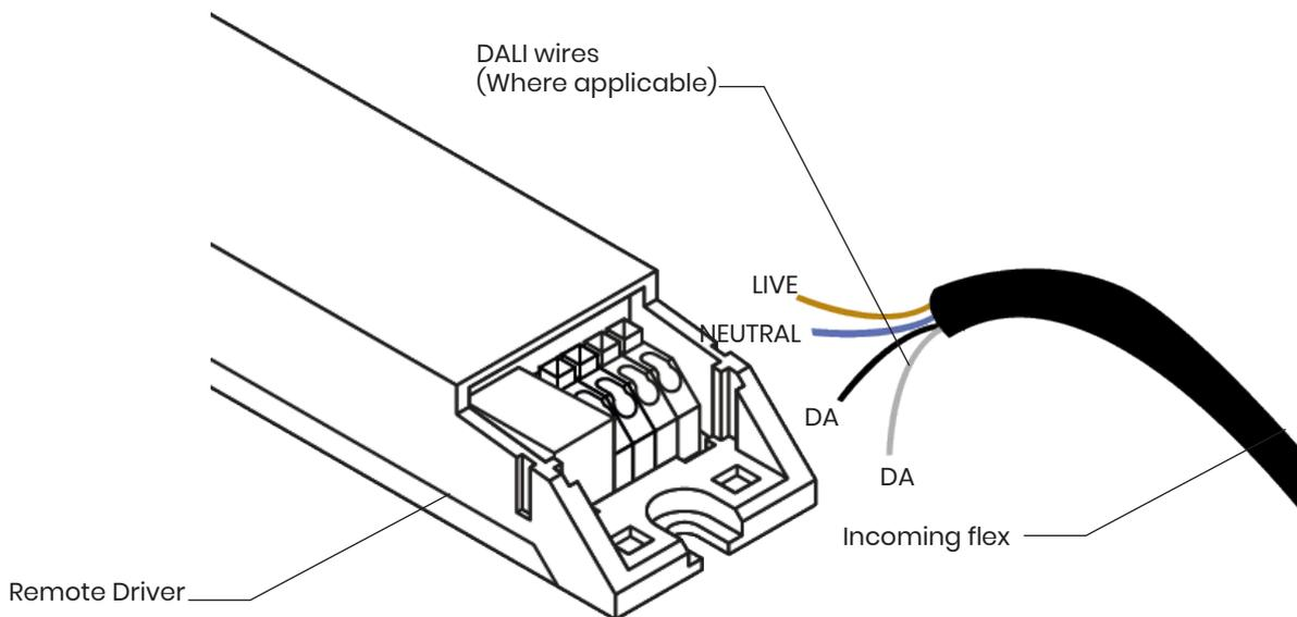
**3** Feed driver through wall cut out.
