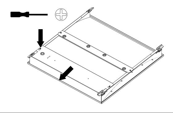
Feed and connect incoming supply (provided by others) to the terminal block (See pages 6 to 8 for wiring diagrams).
