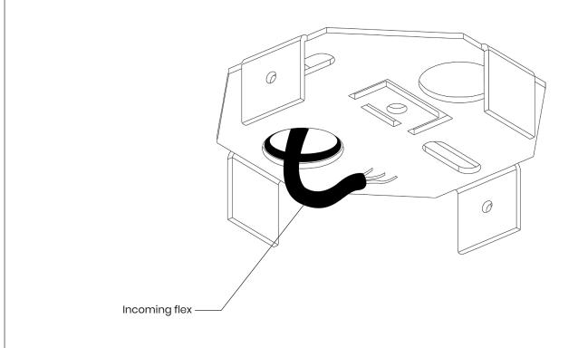
Connect luminaire supply to pre supplied connector blocks.
